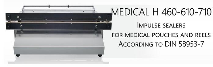
Impulse heat sealers for sealing medical pouches and rolls according to DIN 58953-7. AISI 304 stainless steel cover. Impulse sealing, flat, Sealing height mm 8. Max sealing length mm 460–mm 610–mm 710.
